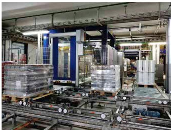
*Safety on the outfeed side is handled with a high-speed sliding door which was installed due to the limited space available in the production.*
