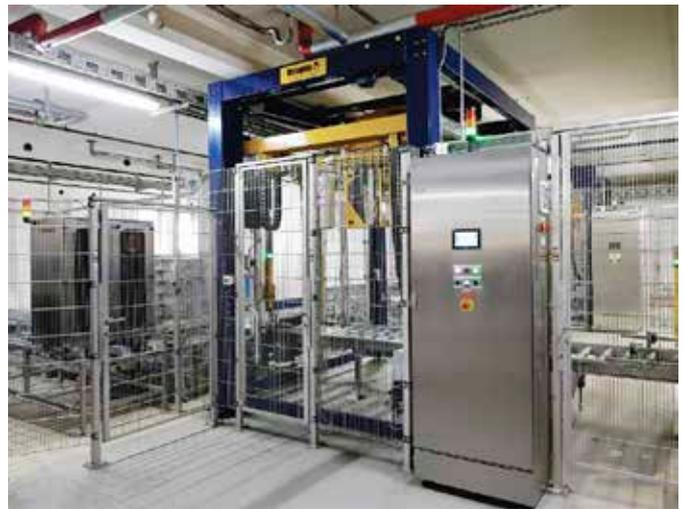
*The first of the two new fully automatic stretch wrapping machines, Octopus 1845S.*
