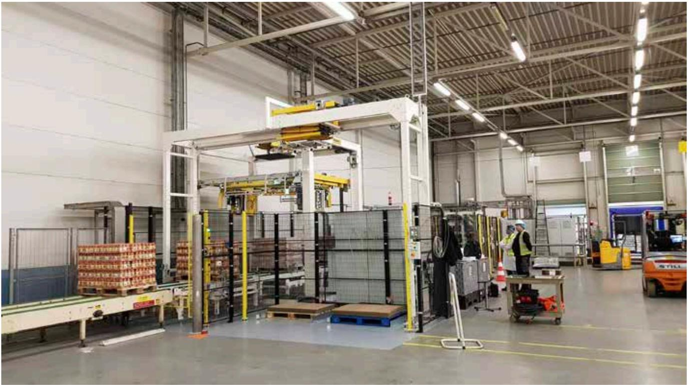
The Octopus 2340T is a twin head machine for higher capacity, equipped with a top cap unit, Automatic Reel Change System (RCS), FlexROPE, pallet lifter and pallet centralizing unit. Haloila also delivered the chain conveyors.
